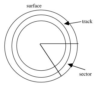
Disk surface: circular disk, coated with magnetic material
