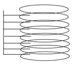
Disk is read via a comb -- 2 read/write "head assembly" at end of each arm (typically, only put disk heads to read inside surfaces, external surfaces are too exposed).
