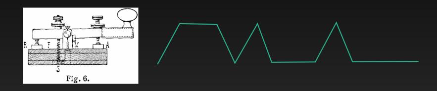
Texts are transmitted as electrical pulses and silence in between Long pulses (1) and short pulses (0)
