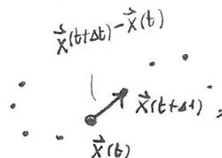
$$\approx \frac{\vec{x}(t+\Delta t) - \vec{x}(t)}{\Delta t} \text{ which is in direction along curve}$$
