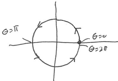
$$\vec{X}(t) = \langle r \cos \omega t, r \sin \omega t \rangle \quad 0 \leq t < \frac{2\pi}{\omega} \quad \text{traces same circle at rate } \omega \text{ rad/sec}$$
