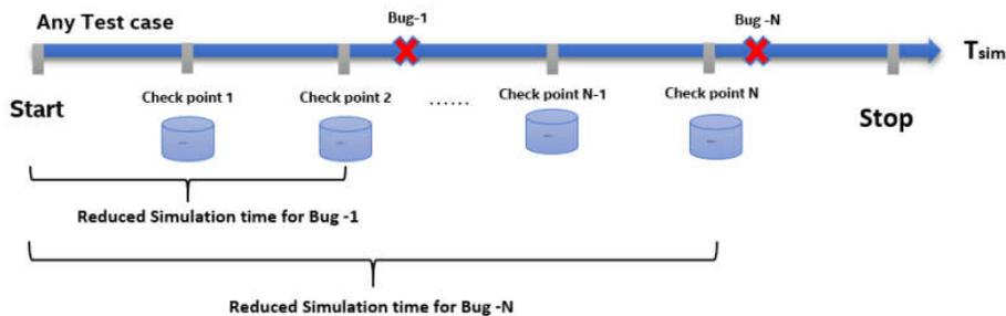
Figure II. Dynamic checkpointing based on clock cycles
