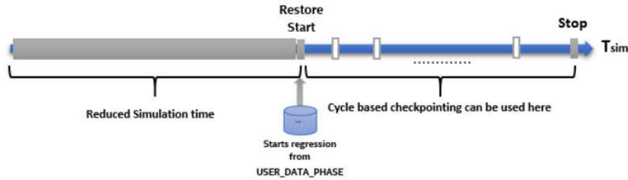
Figure III. Efficient usage of event & cycle based checkpointing
