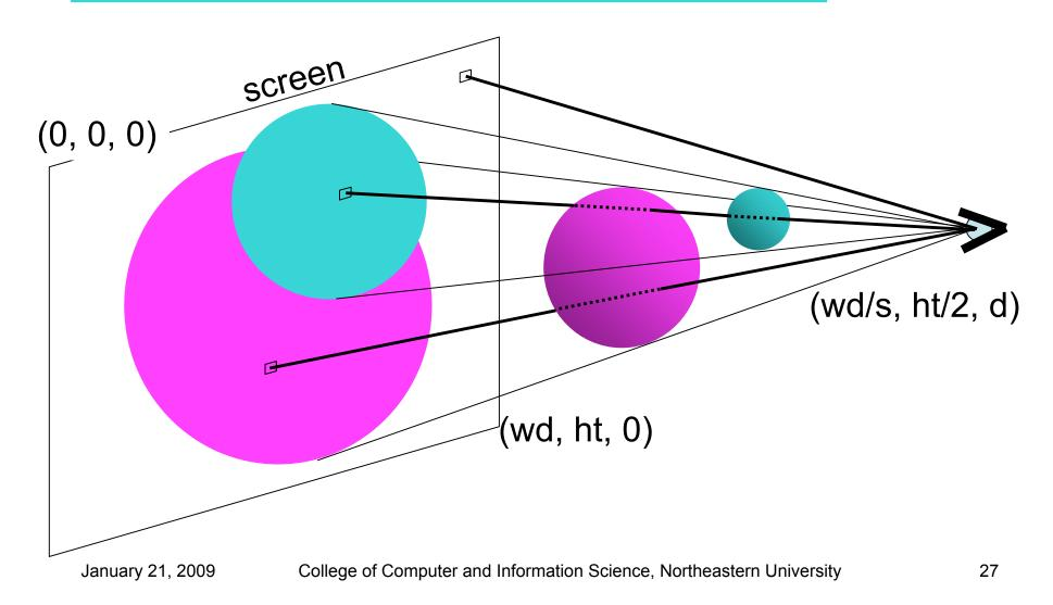
A Viewing System for Ray-Tracing
