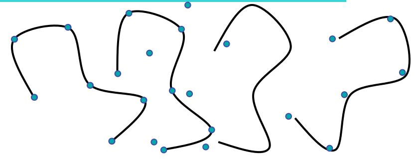
If we rotate the set of control points, we should get the rotated curve.
