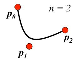
$$n = 2 \quad b_{0,2}(t) = (1 - t)^2 \quad b_{1,2}(t) = 2t (1 - t) \quad b_{2,2}(t) = t^2$$
