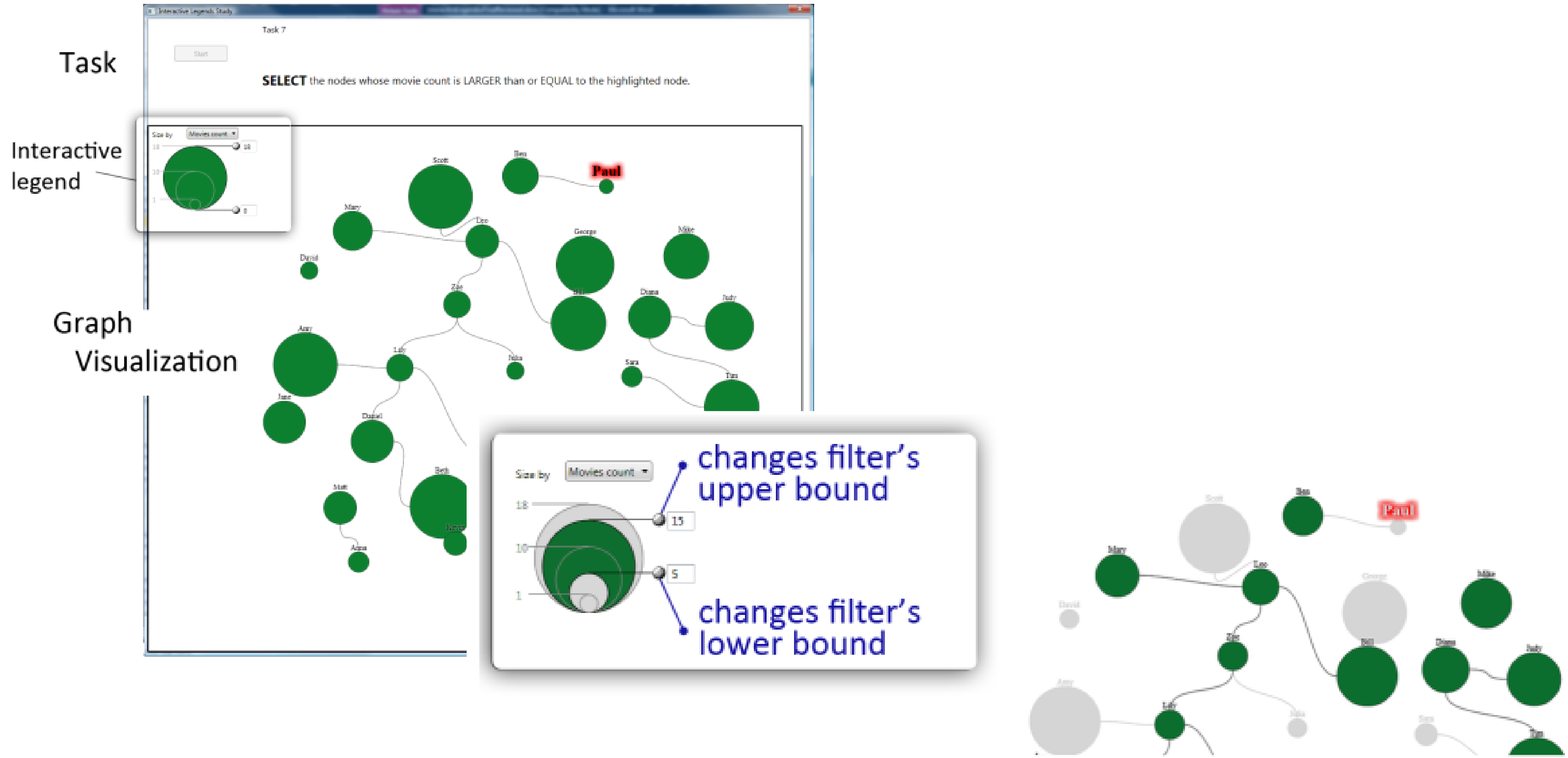
Figure 5: Interactive legend for controlling the size. Handles are provided to filter interactively the visualization.
