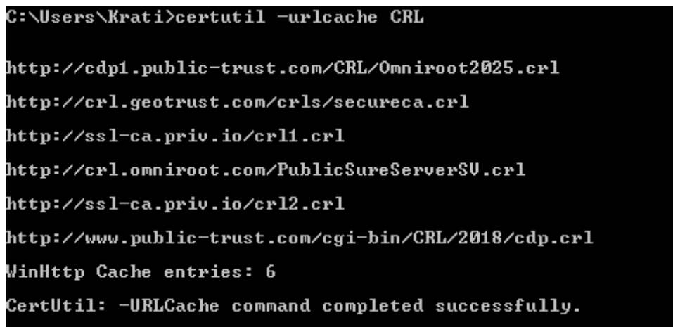
Figure 3.5: Both CRLs from our testbed are cached in Windows after the validation experiment.
