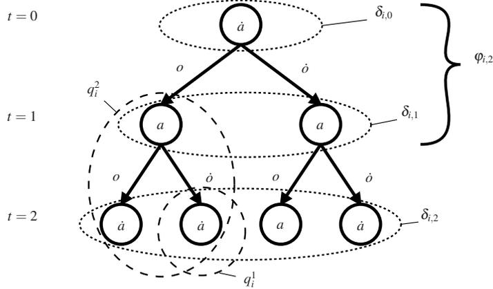
Fig. 4.1: Structure of a policy for an agent with actions  $\{a, \dot{a}\}$  and observations  $\{o, \dot{o}\}$ . A policy  $\pi_i$  can be divided into *decision rules*  $\delta_i$  (which are introduced in Section 4.2.1) or *sub-tree policies*  $q_i$ .
