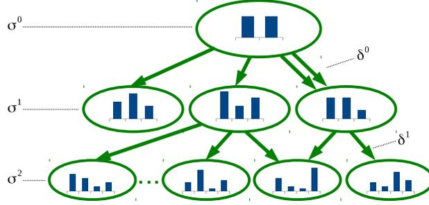
Fig. 4.5: A hypothetical MAA\* search tree based on plan-time sufficient statistics. Illustrated is that two joint decision rules from the root node can map to the same  $\sigma_1$ , and that two  $\delta_1$  (from different  $\sigma_1$ ) can lead to the same  $\sigma_2$ .
