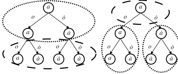
Fig. 4.2: Policy construction in MAA\* (discussed in Section 4.2.2 and shown left) and dynamic programming (shown right). The figure shows how policies are constructed for an agent with two actions  $a, \hat{a}$  and two observations  $o, \hat{o}$ . Dashed components are newly generated, dotted components result from the previous iteration.
