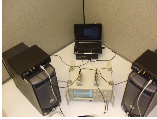
Figure 1: TREKS Test-bed: Two GPU-equipped PCs (Sender and Receiver) and the laptop (Jammer) individually connected to USRPs.
