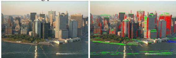
Previous work and our experiments indicate that this algorithm is prone to failures and errors in some cases: spurious edges, Canny thresholds and vanishing points approaching infinity leading to precision errors. When this occurs, we revert to a manual approach: the user select three pairs of parallel lines that are mutually perpendicular to each other. These pairs give the three vanishing points.
