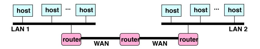
LAN 1 and LAN 2 might be completely different, totally incompatible LANs (e.g., Ethernet, Wi-Fi, ATM, Circuit-switched)
