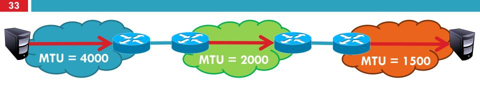
Length = 2000, M = 1Offset = 0 IP Data 20 1980 Length = 1840, M = 0Offset = 1980 IP Data 20 1820
