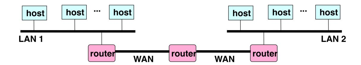
LAN 1 and LAN 2 might be completely different, totally incompatible LANs (e.g., Ethernet, Wi-Fi, ATM, Circuit-switched)
