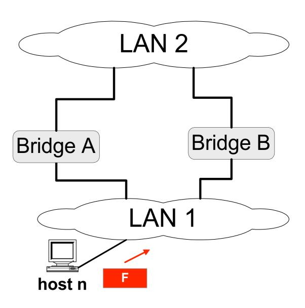
Consider the two LANs that are connected by two bridges.
