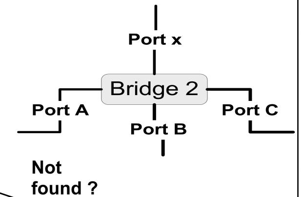
Flood the frame, i.e., send the frame on all ports except port x.
