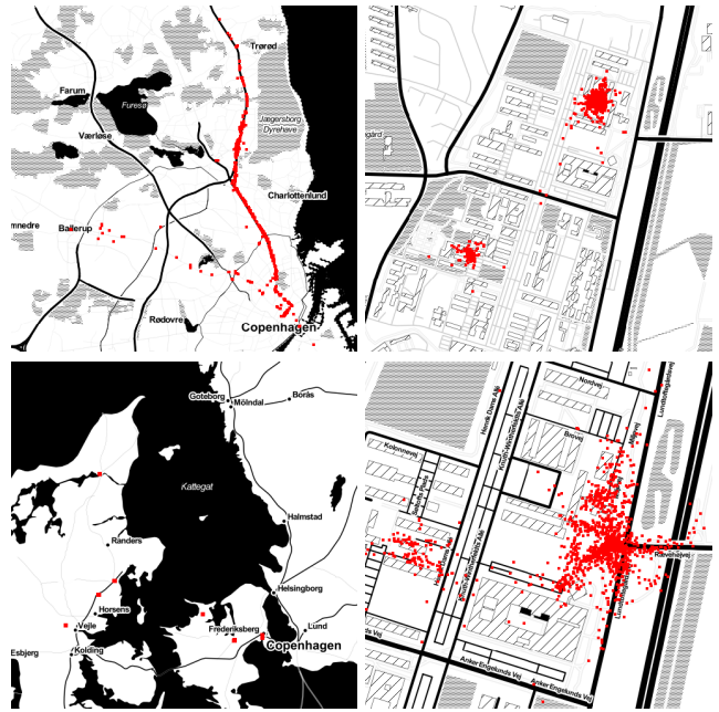
Figure 4: Longitudinal observations reveals mobile and moved APs. Shown are the observed locations of a mobile AP installed on a bus (top left), an moved AP (top right), an AP moved 6 times (bottom left), and an AP with ambiguous behavior (bottom right).
