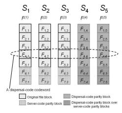
Figure 1: Encoding of file F: on the left, original file represented as a matrix; on the right, encoded file with parity blocks added for both the server and dispersal codes.
