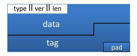
Browser side  $Enc(k_{b\rightarrow s}, data, ctr_{b\rightarrow s})$ : Step 1: tag  $\leftarrow Tag(k_{mac}, [++ctr_{b\rightarrow s}] \parallel header \parallel data])$ Step 2: pad [ header || data || tag ] to AES block size Step 3: CBC encrypt with  $k_{enc}$  and new random IV Step 4: prepend header
