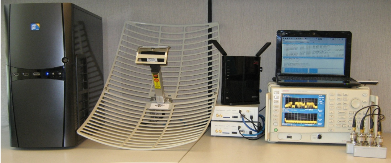
Figure 5. Overview of hardware used in the prototype implementation of the attack. From left: desktop, antenna, router, USRP2 software-defined radio, victim client, signal analyzer (for evaluation), and attenuators.
