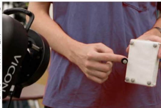
Figure 3. Brick model with 5 retroreflective markers
