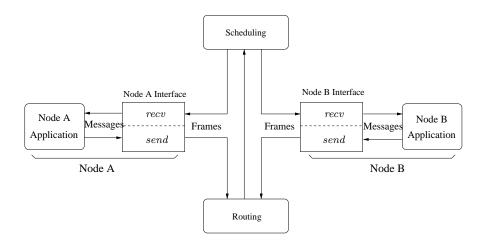
Figure 2: GeNoC: A generic network on chip model
